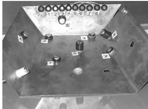
Fig. 1. Positioning task. This task requires touching the top of eight cylinders (in varying three-dimensional positions) with the tip of the minimally invasive surgery (MIS) instrument. A correctly touched cylinder results in the lighting up of a lamp (above in the picture) corresponding to this cylinder.
