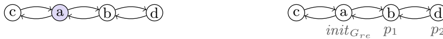
Fig. 9 Running example: the topology G_{re} and the graph LTS G_{re}|\bar{g} for \bar{g} = (b, d) . The 2-topology G_{re} with T_1 = \{a\} and T_2 = \{b, c, d\} is depicted to the left. The graph LTS G_{re}|\bar{g} is depicted to the right.
