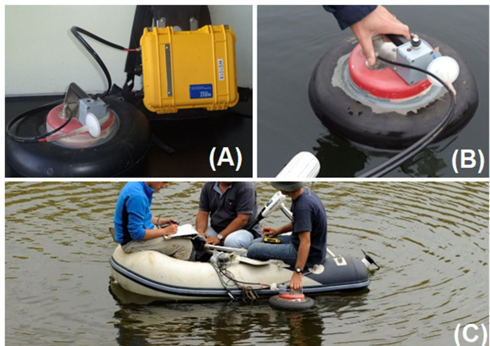
Fig. 2 (A) Portable CO 2 flux instrument + modified accumulation chamber. (B) Floating accumulation chamber. (C) Measurements at the water surface, using the modified accumulation chamber method.
