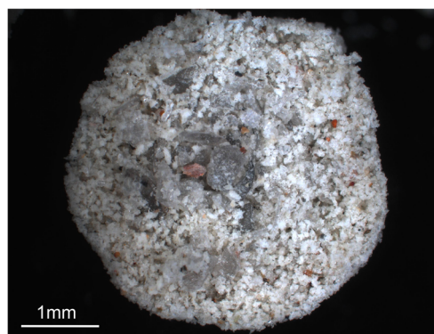
Fig. 11 Artificial ash aggregate (AP2) produced of an initial PSD < 500 \mu\text{m} . Particles of several 100 \mu\text{m} are centered in the core region of the aggregate; the rim is built out of finer material. The aggregates show a heterogeneous distribution of particle packing of residual inter-clast pore space
