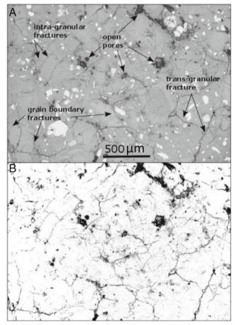
**Fig. 1** a Scanning electron microscope backscatter photomicrograph of a sample of intact dacite showing a pervasive microfracture network with no obvious or preferred orientation. Large and small isolated pores are also present in the sample and are labeled on the image. Microstructural elements are labeled respectively. Image was taken in the *XY* plane (perpendicular to fluid flow). **b** Corresponding binary image of the SEM image converted using ImageJ. *Black areas* represent porosity
