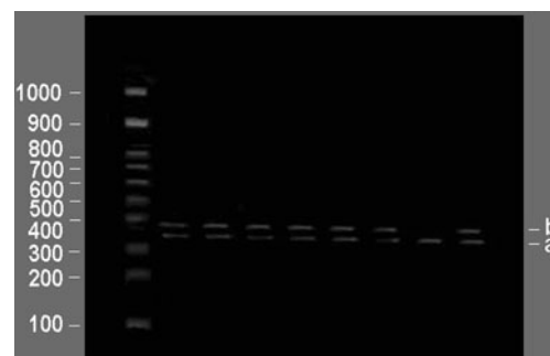
Fig. 4 PCR results showing diagnostic bands at 350-bp for Babesia (a) and 370bp for Theileria (b). Lane M 100-bp ladder=DNA marker (from Fermentas, Germany)
