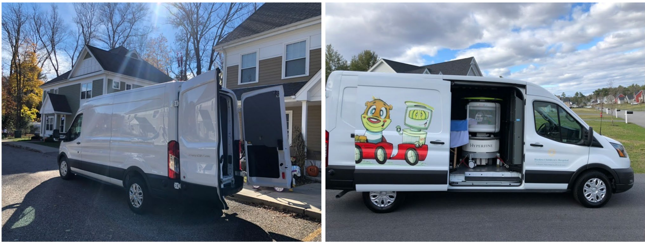
Fig. 1 Example photos of the Scan-Van at participant homes. Participants enter the van from the rear doors. The side door can be opened to reduce claustrophobia, allow extra cooling, or just improve the general participant experience
