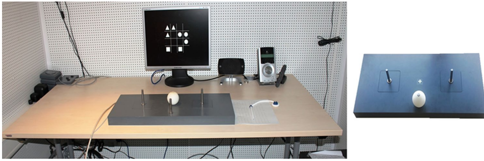
Fig. 1 Experimental set-up (left) and task board (right). In the figure, the experimental set-up shows the example stimulus and answer sheet for the visuospatial task. The task board consisted of three sticks as the start position and two motor targets (left and right). A yellow
