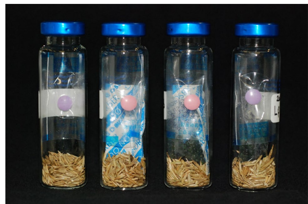
Fig. 2 Photograph showing the experimental set up. 20 mL glass headspace vials were filled with 1 g of seeds (seeds pictured are Lolium perenne ) which had been equilibrated to 60% RH. Control vials (left) contained just seeds and an oxygen indicating tablet, which was blue/purple in the presence of oxygen ( >0.5\% ) and turned to pink when oxygen levels were <0.1\% . Other vials (second from left to right) contained seeds, an oxygen indicating tablet and either a 20 cc oxygen absorber ( \text{O}_2 absorber), a 20 cc oxygen absorber and a silica gel sachet ( \text{O}_2 absorber + silica), or a silica gel sachet which had been pre-equilibrated to 60% RH (silica). All vials were sealed with PTFE-lined crimp seals
