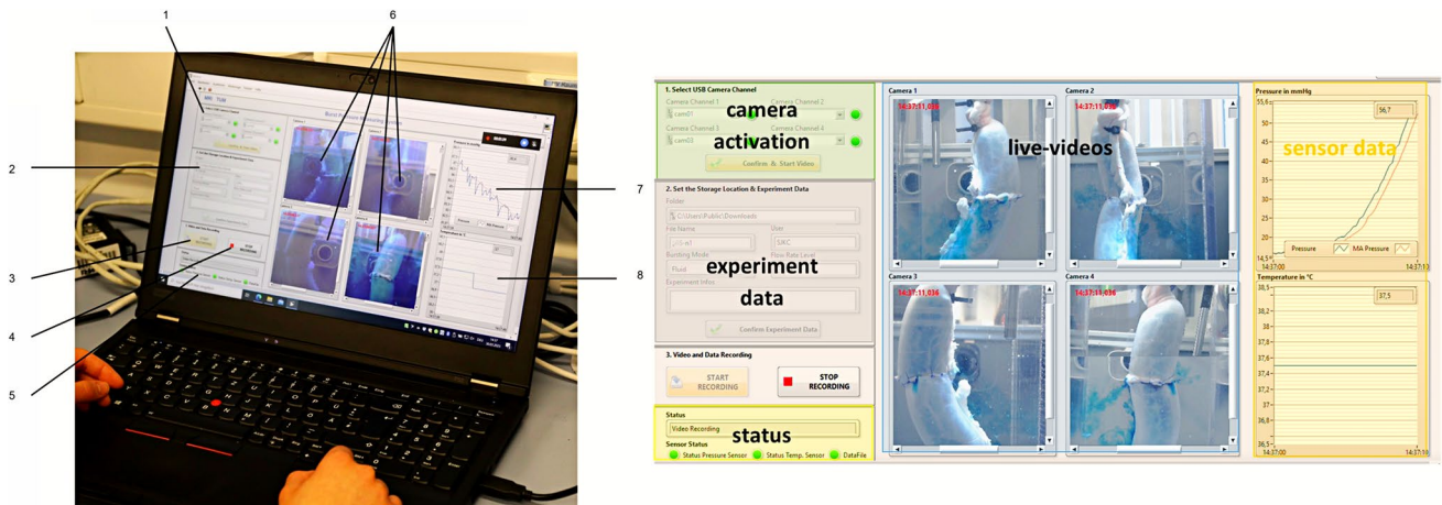
Fig. 3 Human machine interface (computer) during an experiment. The figure displays the HMI on a computer used during the experiment. 1=Camera activation: allows the user to activate the cameras for recording; 2=Enter experimental data: enables inputting relevant experimental data; 3=Start recording of the experiment: initiates the recording of the experiment; 4=Stop recording of the experiment:
