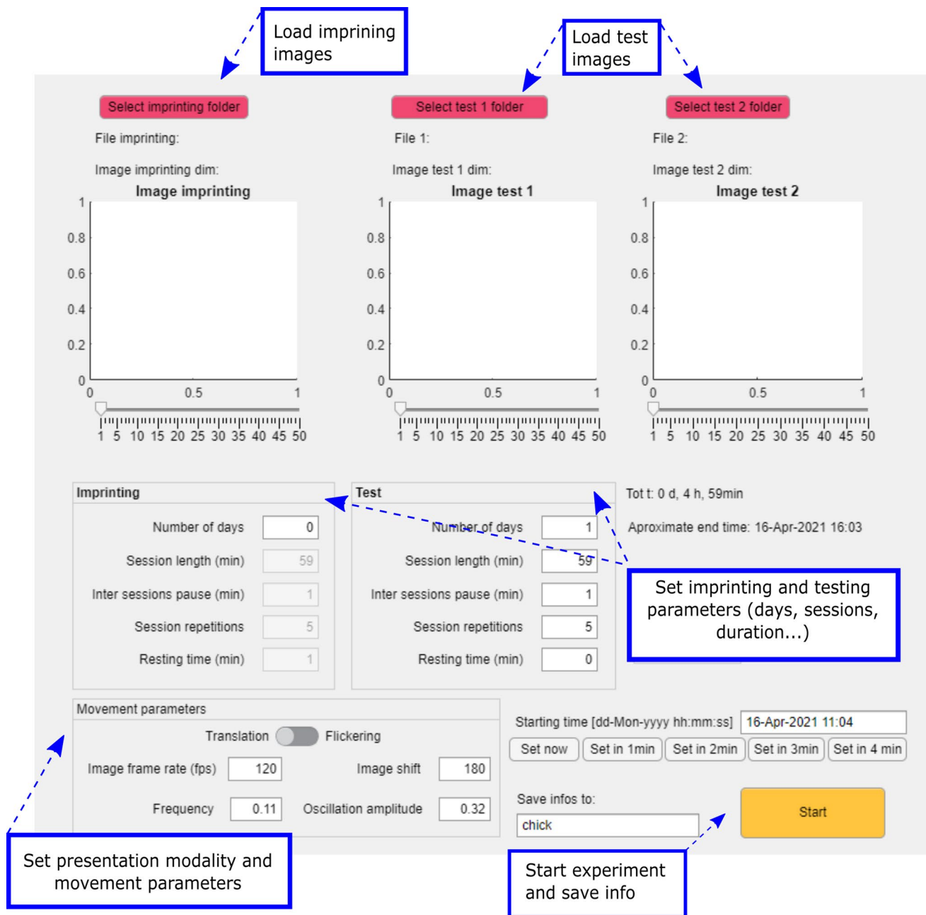
Fig. 2 ImprintSchedule graphic user interface. Different parameters of image presentation can be set, such as the duration of image appearance (divided into days and sessions) both in the imprinting
