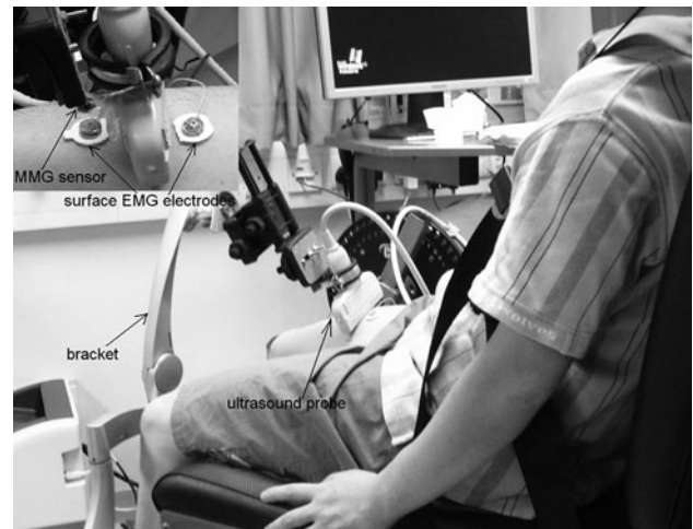
Fig. 1 Experimental setup for collecting EMG, MMG and ultrasound images from the subject's right rectus femoris (RF) muscle during isometric ramp contraction. The ultrasound probe was aligned perpendicularly to the RF muscle belly using a multi-degree adjustable bracket. The two surface EMG electrodes were located at the two sides of the ultrasound transducer and in parallel with the muscle fibers. The MMG sensor was placed as near as possible to the distal EMG electrode, and they were in parallel with the ultrasound probe
