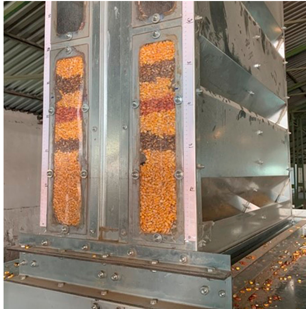
Fig. 10 Coloured particle stripes in the model dryer apparatus
