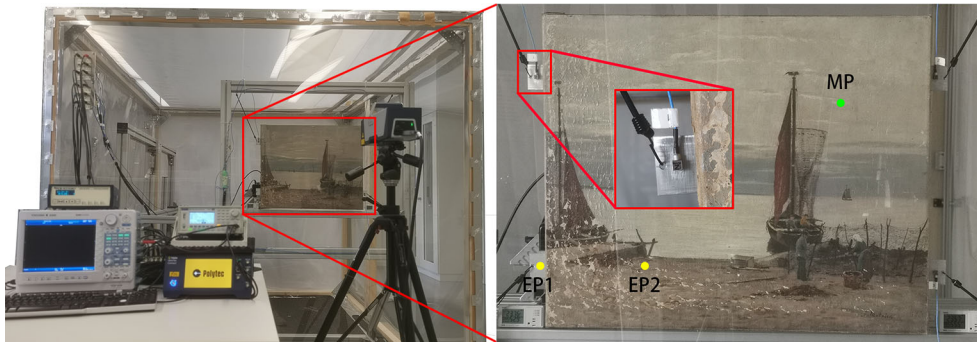
Fig. 2 Experimental setup for the tested painting in a climate box with approximately free suspension
