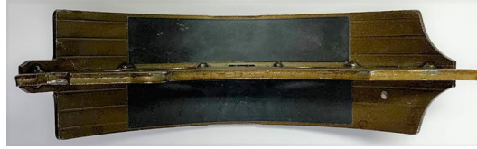
Fig. 5 Industrial brake shoe attached with shims as investigated in [17]
