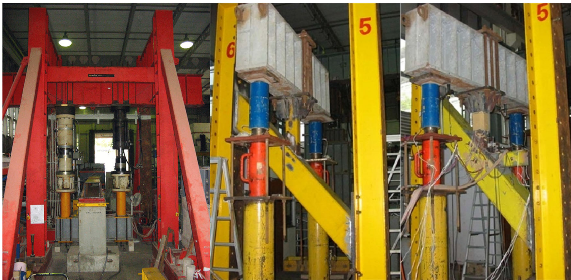
Fig. 6 The experimental test rigs for cracked SHS T-, Y- and K-joints
