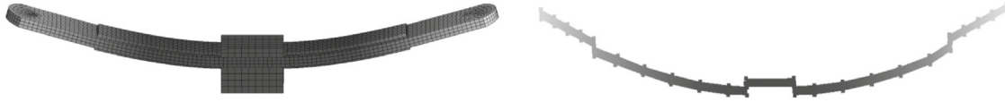
Fig. 7 1st bending mode of the finite element model ( left ) and the experimental modal analysis ( right ) at 167 Hz
