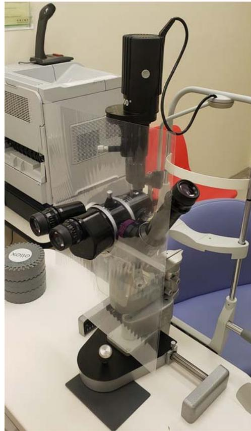
**Fig. 3** Protective shield installed on a slit lamp
