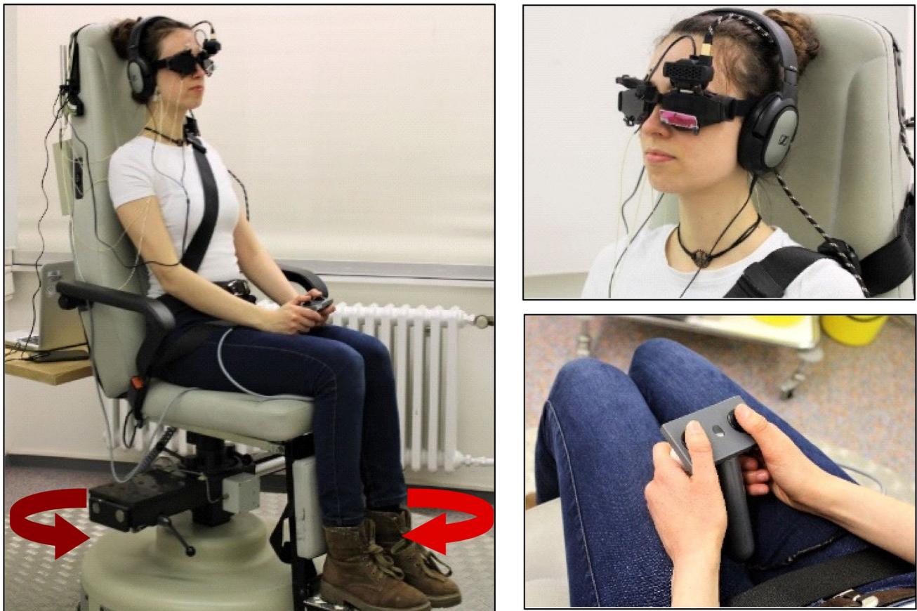
Fig. 1 Vestibular perception threshold of chair rotation. The subject was sitting on the vestibular chair, refrained from visual and acoustic signals (see methods). The vestibular stimulus (chair rotation around the earth-vertical axis) was moving with a constant acceleration in an unpredictable direction, being randomized before (acceleration of 0.3^\circ/s^2 ). The subjects were asked to indicate the onset of passive egomotion perception by a response button once they were certain
