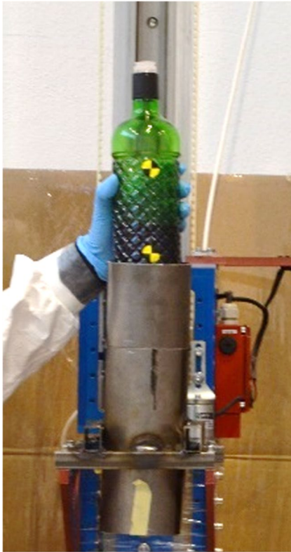
Fig. 2 Metallic cylinder where the bottle was placed for the free-fall impacts
