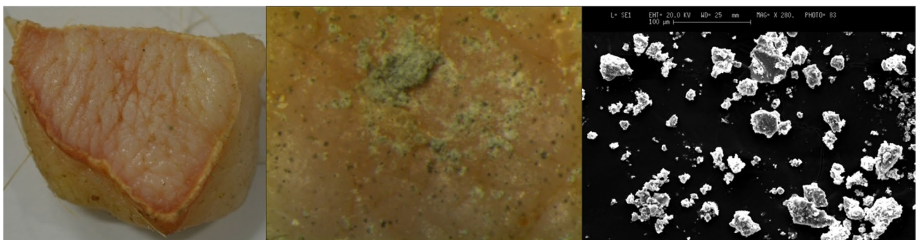
Fig. 8 Image of the skin sample placed exposed in the construction site and the particulate present on it. The debris is observed through the episcopic microscope (16X) (in the middle) and SEM (on the right)
