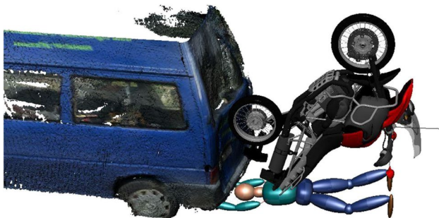
Fig. 12 Hypothetical compression of the PTW rider between the PTW and the asphalt
