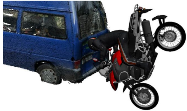
Fig. 9 Collision position, which is compatible with the available data. Note that this illustration does not show the type of motorcycle used in the present case
