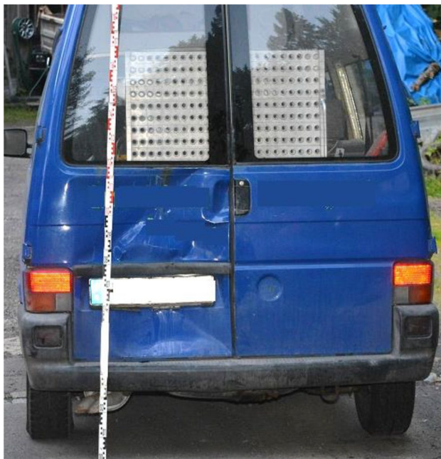
Fig. 5 Deformations of the left rear door
