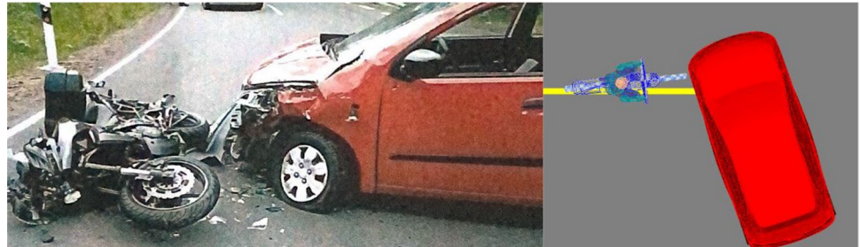
Fig. 3 End positions of the vehicles (left), collision position in PC-Crash (right)
