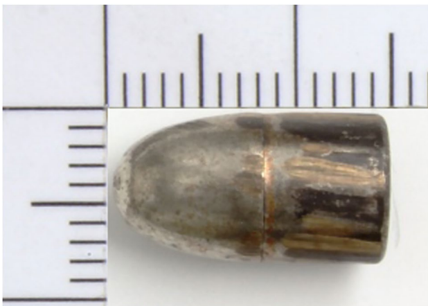
Fig. 1 The bullet retrieved from the passenger door sill. Ultimately, this bullet could be attributed to the tangential shot. The bullet was undamaged, apart from the typical grooves left by the pistol barrel
