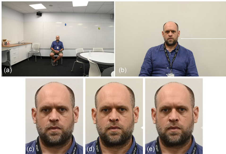
Fig. 6 Images of the same subject taken using the same Nikon® D780 24.5-megapixel camera at the same focus distance (3.5 m), but with at two different focal lengths (24 and 120 mm on an AF-S NIKKOR® 24–120-mm 1:4G lens) to show that the perspective distortion is set by the focus distance, not set by the lens/its focal length. As the focus distance has not been changed, after fixed aspect ratio resizing of the image taken with the shorter focal length lens, the two faces precisely superimpose. a Raw image produced by the macro 24-mm
