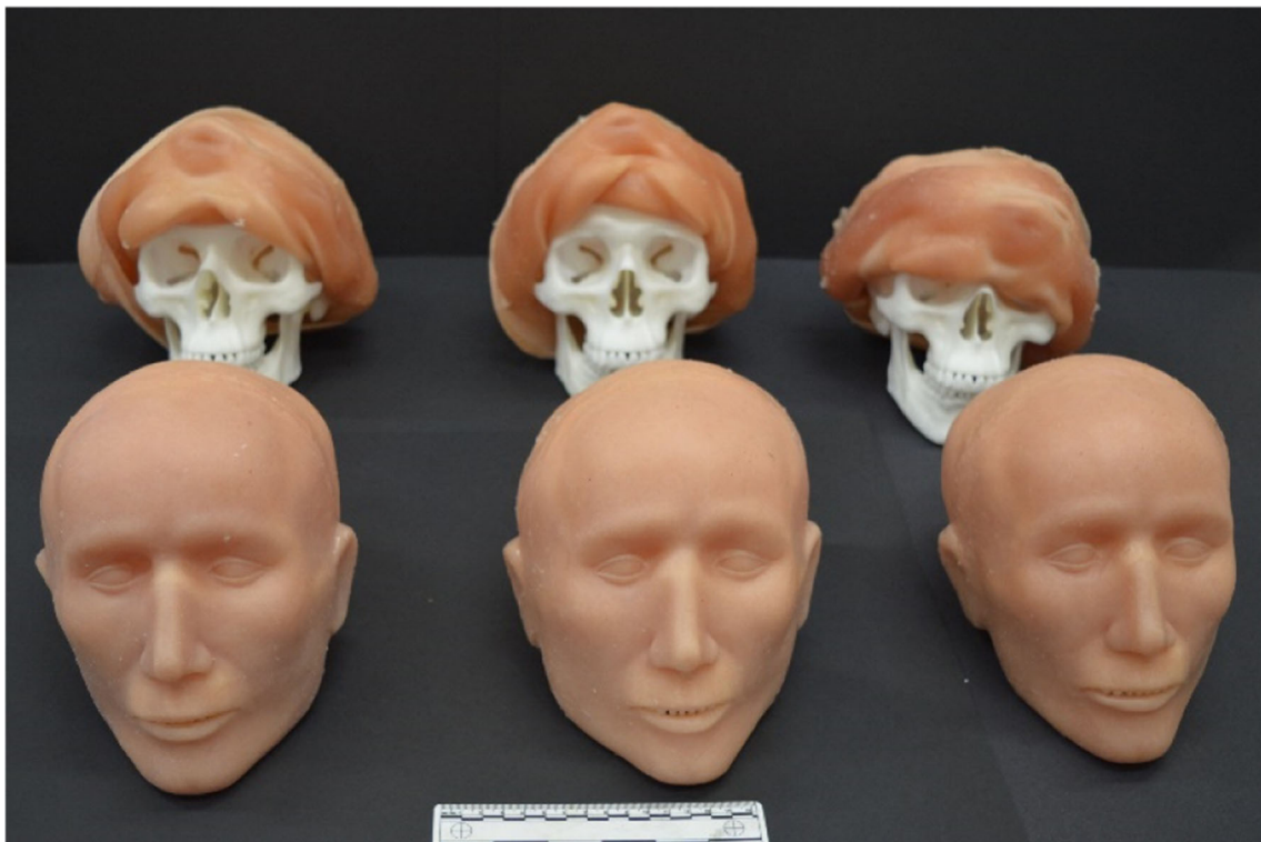
Fig. 2 MU51 polymer skulls with moulded PDMS faces and scalps
