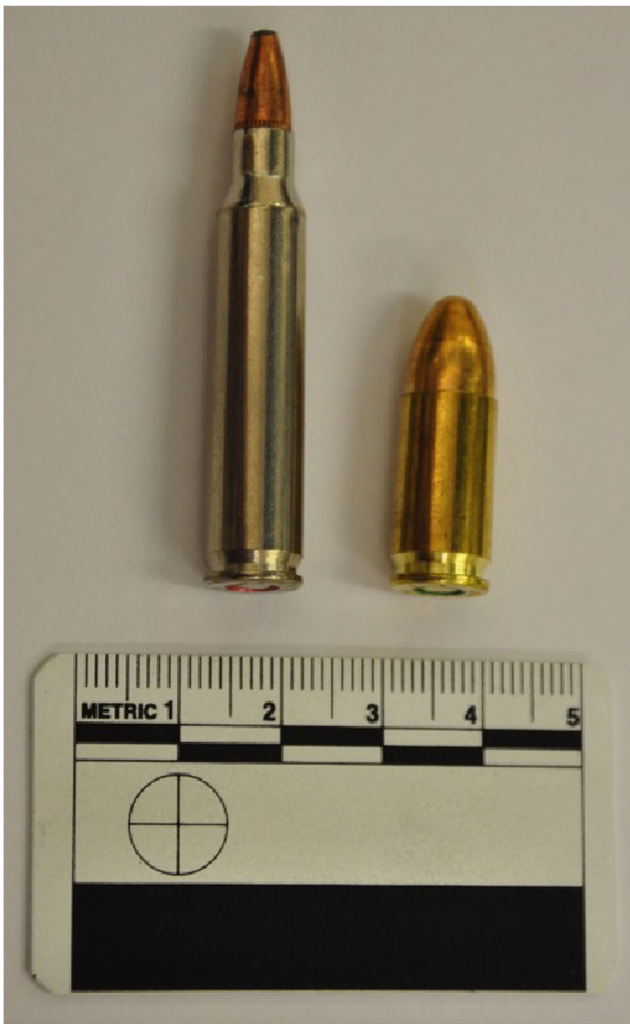
Fig. 1 .223 Remington (5.56 × 45; 62 grain; Federal Premium® Tactical® Bonded®) (left) and 9 mm Luger (9 × 19 FMJ; 124 grain; DM11 A1B2) (right)
