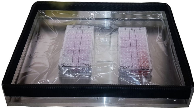
Fig. 1 A photograph of an acrylic chamber covered with a plastic pouch. The chamber can be filled with mixed gases through a narrow hole made in one side of the chamber. The side dimensions of the chamber are 30×30 cm
