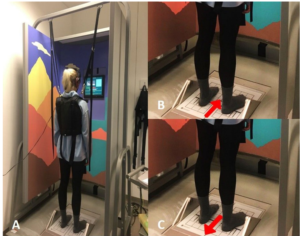
Fig. 1 A Computerized static balance test system. The participant is wearing the headphones of experiment 2. B As an example, the setting of the Motor Control Test (MCT) is shown, here forward translation: C backward translation of the MCT
