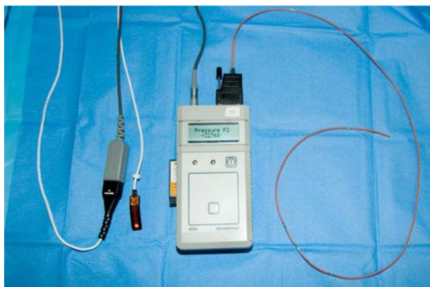
Fig. 1 The ApneaGraph device with its components: a pulse oximetry probe and the fine-bore nasal catheter with four transducers
