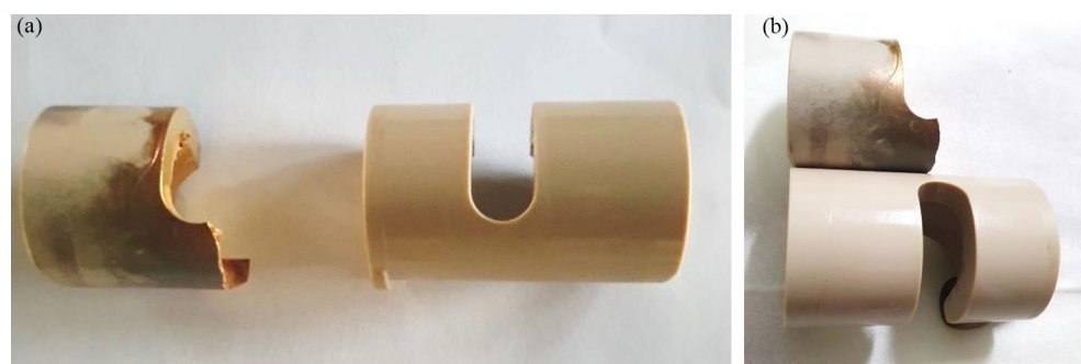
Fig. 2 Figure 2a illustrates a side-by-side view of the broken PEEK component compared to the original. Figure 2b illustrates one above the other emphasizing the fracture location as compared to the complete one. The failure occurred at the point of impact during full extension, at the root of the semicircle, where the metal post impacts the PEEK
