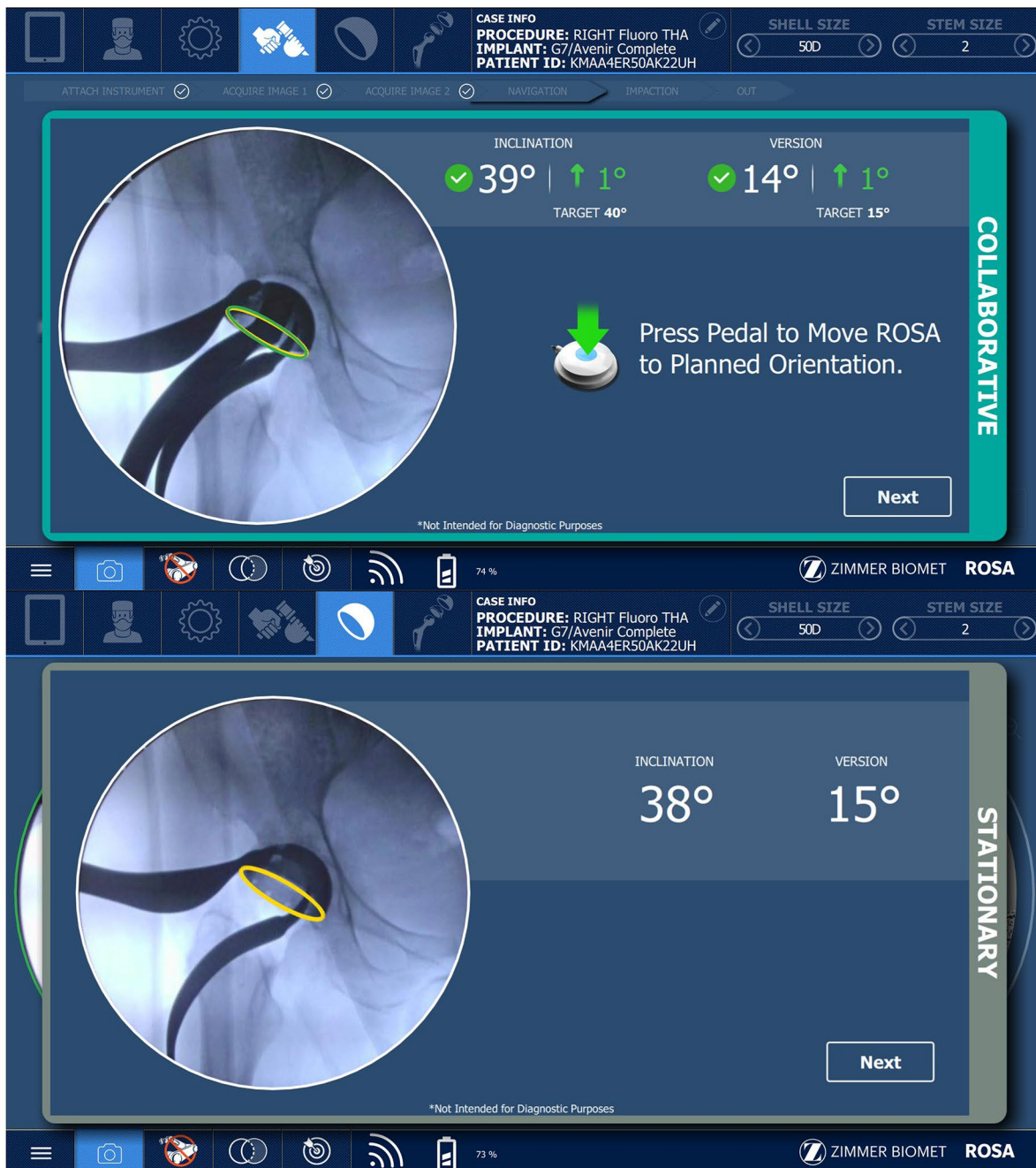
Fig. 2 An overview of the intra-operative navigation interface of the ROSA® Hip System. (Top) Screenshot of Cup Impaction panel. (Bottom) Screenshot of Cup Verification panel
