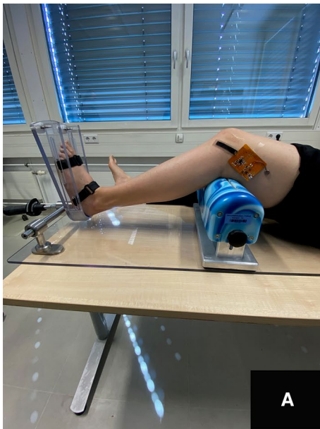
Fig. 2 Positioning of the strain sensor in the course of the ALL and internal rotation of the lower leg with a torque of 2 Nm; the strain sensor was glued in the course of the anterolateral ligament below the lateral epicondyle of the femur to Gerdy's tubercle
