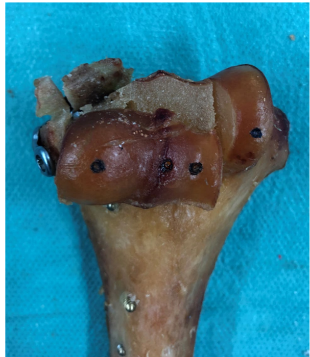
Fig. 4 Anterior view of a group PLP specimen after cyclic loading and load to failure testing with the capitulum fragment's proximal displacement
