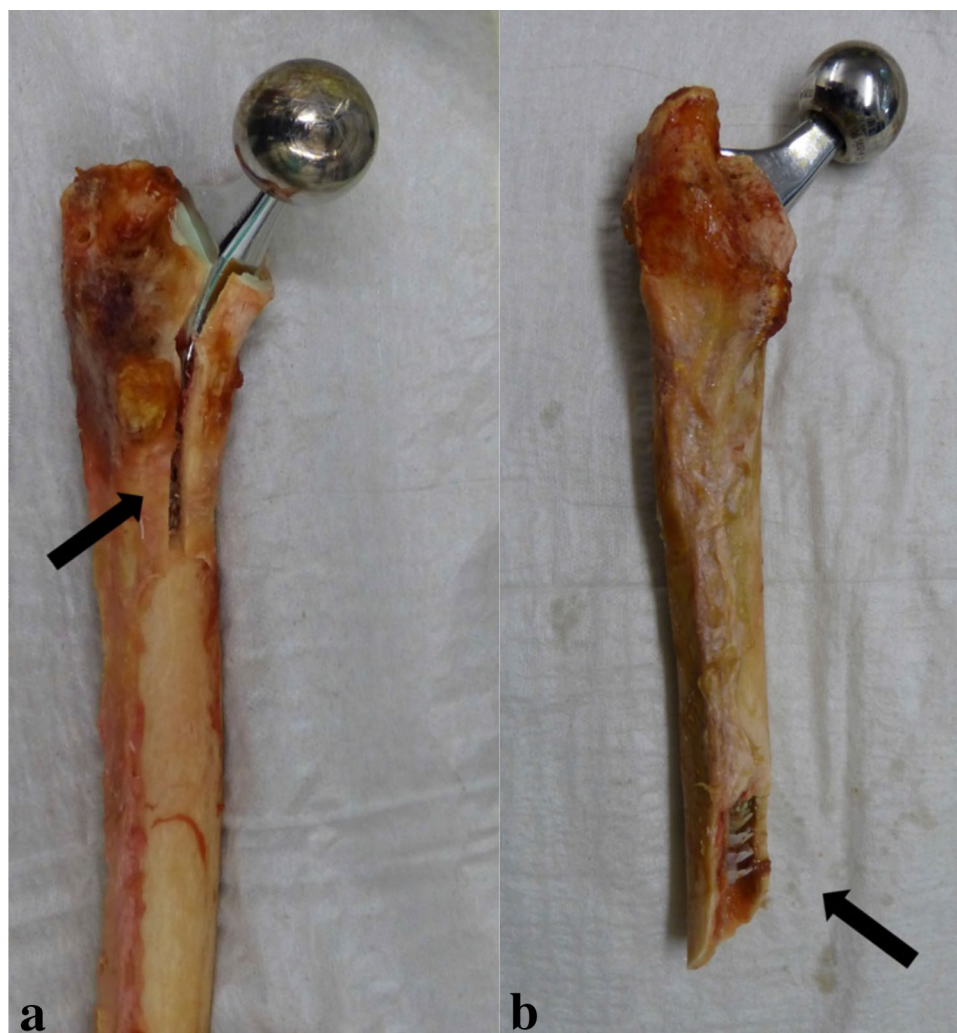
Fig. 3 a, b Fracture pattern of periprosthetic fractures induced in both groups. All short stems showed proximal fractures according to Vancouver type B3 (a), 4 out of 6 straight stems showed Vancouver type C fractures (b)
