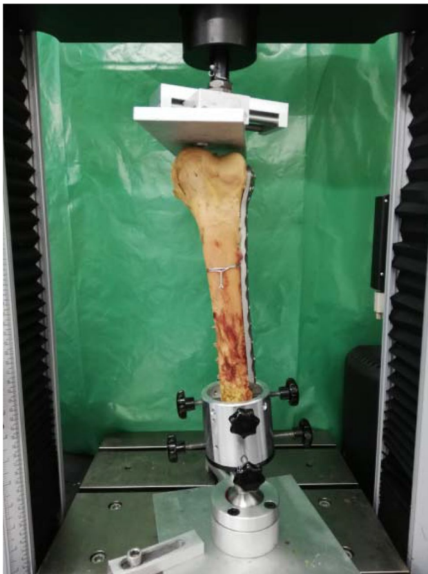
Fig. 4 Test setup demonstrating force application with a metal plate movable in two directions. The femoral shaft was statically fixed in an anatomical 5–7° valgus position. Force was applied in a retrograde manner
