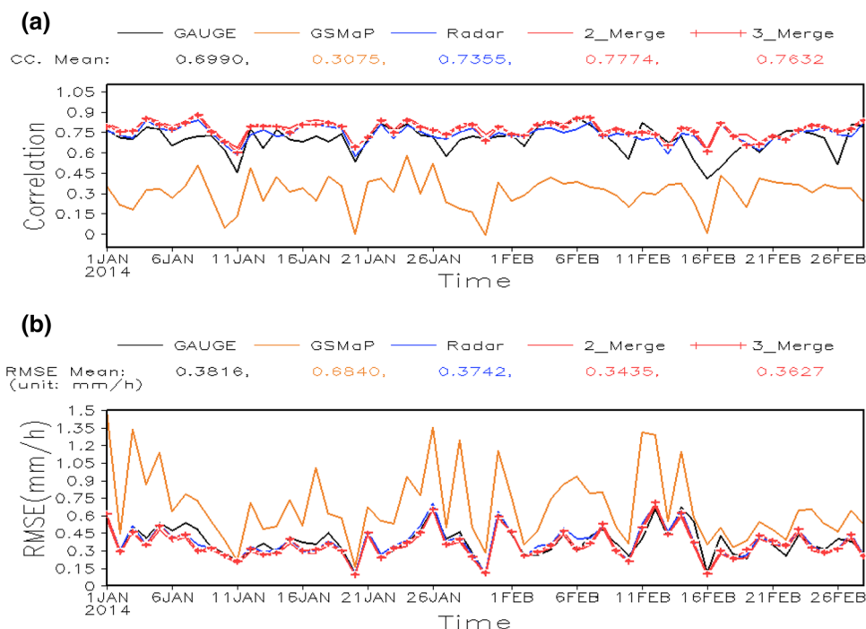
Fig. 7 Time series of daily data errors represented by a CC and b RMSE (mm/h) of 3_Merge (red line with plus sign), 2_Merge (red line), radar (blue), satellite (orange) and gauge (black) analysis data from January–February 2014 for the independent test. The time mean values of CC and RMSE respectively for each analysis are shown in the legends
