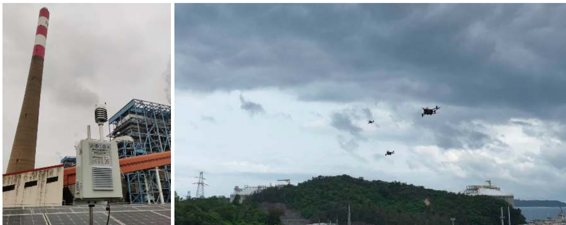
Fig. 2. Photos of the campaign in Shenzhen. The left-hand panel shows the ground-based station near the power plant, with an NDIR sensor in the enclosure. The right-hand panel shows a swarm of drones for coordinated observation.
