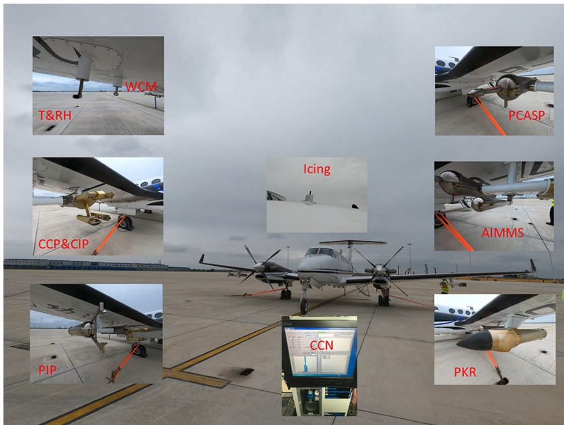
Fig. 5. Photos of the Shanxi KingAir aircraft probes and onboard Ka-band cloud radar (PKR).
