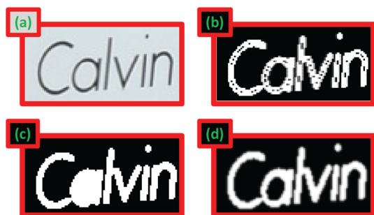
Fig. 8 a Original image for color detection, b gradients of original image, c after flood fill of the gradients, and d after background color elimination
