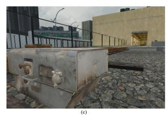
**Fig. 1** An virtual environment for shunting training. **a** The workshop area. **b** A railway outside the workshop. **c** A point machine located beside the railway for switching the direction of the rail
