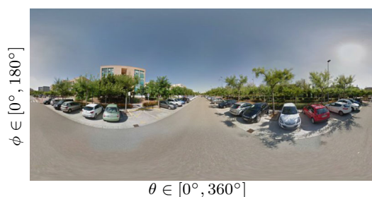
Fig. 2 Panoramic view. The entire spherical image is displayed on a plane. Each coordinate represents an angle (\theta, \phi) , which jointly identify any point in the sphere
