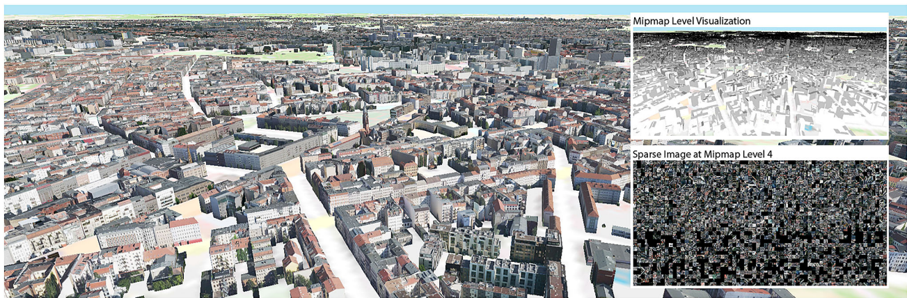
Fig. 5 Rendering of the Berlin city dataset. 13.7K texture mipmaps are loaded and cached in the sparse image at a rate of 56.6MB/s. Top inset: the resolutions of loaded texture mipmaps are visualized as grayscale
