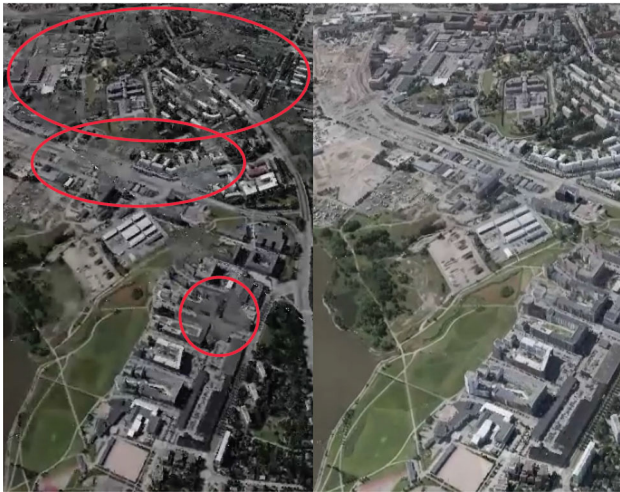
Fig. 8 Comparison of rendering quality during texture streaming between unity (left) and our method (right). In unity, texture pop-ins are visible as low resolution mipmaps are immediately refined into high-resolution ones. In our method, we refine mipmaps at all levels using our mipmap blending method and adaptive algorithms, resulting in less texture pop-ins and more uniform texture resolutions
