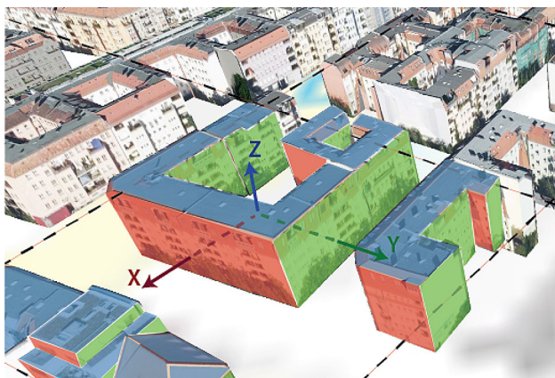
Fig. 2 An illustration of our mesh clustering scheme to generate texture atlases for a city dataset. The black dotted lines indicate uniform rectangular grid regions. The red, green, and blue arrows are globally aligned axis. Within each grid region, building meshes are separated into six orientation groups based on their closest normals alignment to the global axis. Back faces are grouped but not illustrated
