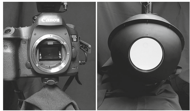
Fig. 2 Camera under test (Canon 5D Mark III) and the integrating sphere. To ensure each pixel receives light from the whole disk-shaped illumination source (the integrating sphere output port), an f-number of 8 is required. By placing the sensor at a distance D of 81.28 cm from the output port having a diameter d of 10.16 cm, an f-number of 8 is achieved, where f_{\#} = d/D
