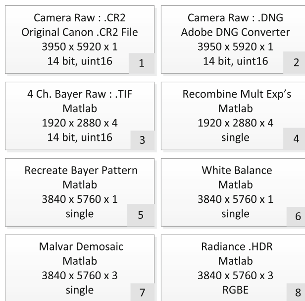
Fig. 5 Processing Blocks illustrating the 8 key processing steps of the recombination procedure. Blocks 1–3 are single capture process and Blocks 4–8 describe the recombination process
