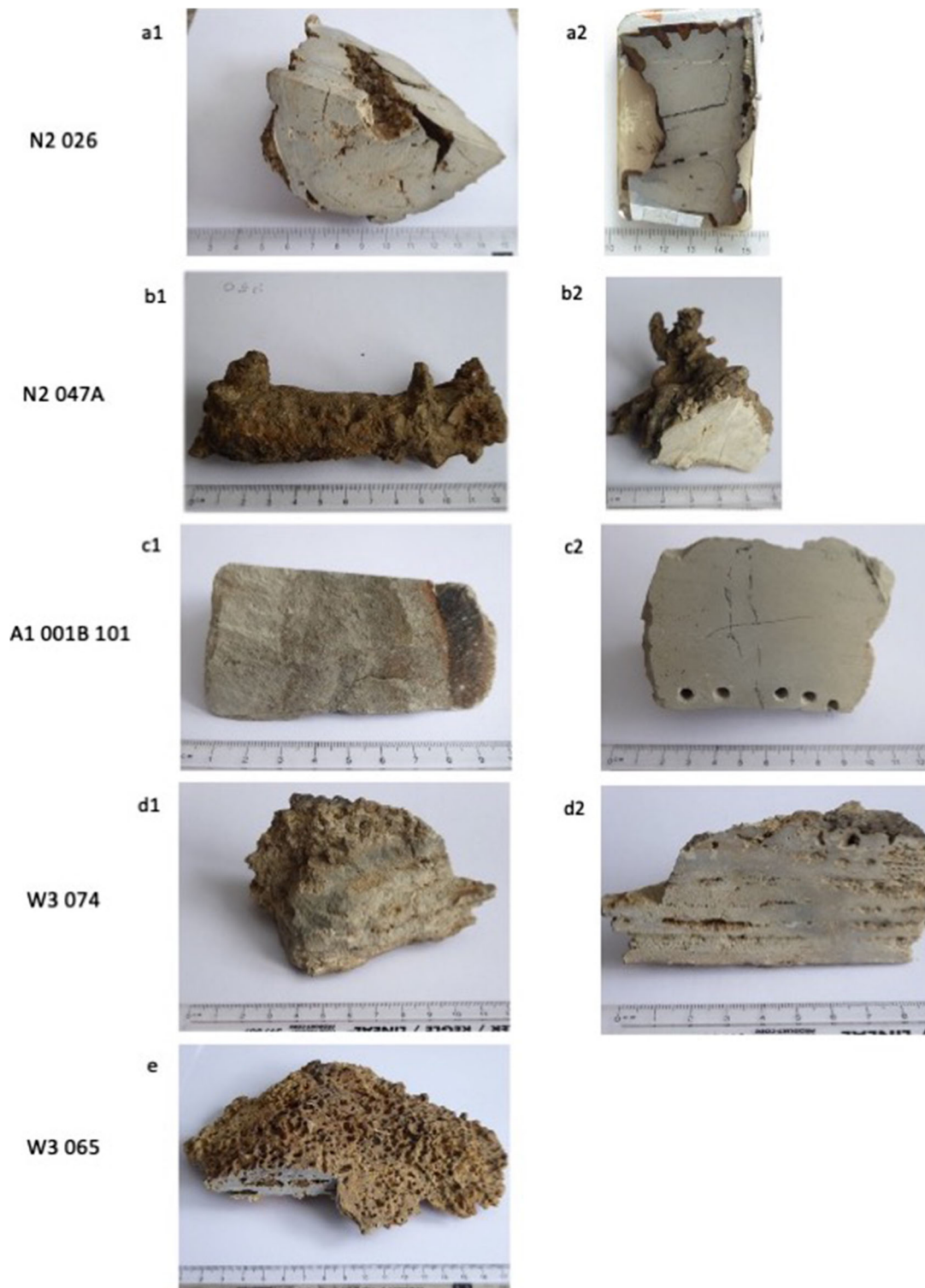
Fig. 4 Photographs of representative carbonate structures from the Palmachim disturbance. The respective data are given in Table 1. a Area N2, parts of sample 026 Chimney. (a1) The lower part of the chimney having a conical shape, a central conduit, and transverse partitions. (a2) Slice of the upper part from which 22 aliquots were analysed. b Area N2 sample 47A branch. (b1) The sample has an irregular elongated shape. (b2) Side view of a cut surface showing a dense massive texture. c Area A1 sample 001B 101 wedge. (c1) Side view reveals layers,
