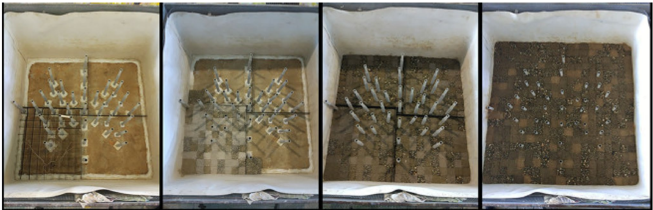
Fig. 4 Illustration (from left to right) depicting the sequence that forms the layers of cells constituting the geological formation. Reproduced with permission from Brunetti et al. [32], (adapted from Figure 2 of the original article)
