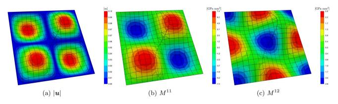
Fig. 6 Deformed configuration for the laminate in Fig. 4a with superimposed mesh grid and contour of the magnitude of the displacement (a), generalized moments  $M^{11}$  (b), and  $M^{12}$  (c)
