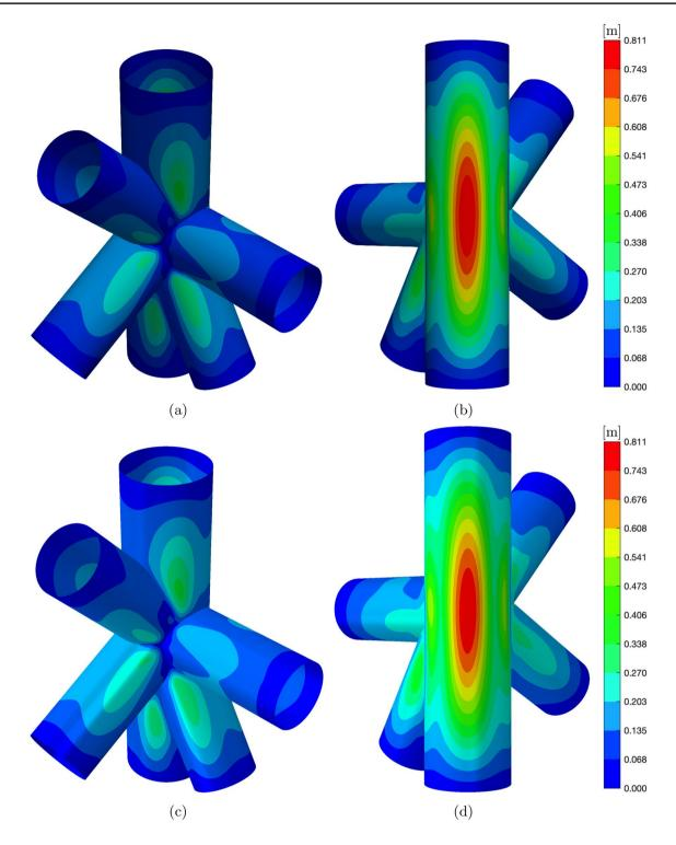
Fig. 14 Two different views of the contour of the magnitude of the displacement for the structure described in Sect. 5.3 obtained with the method presented here (a) and (b), and with the elements STRI3 in  $Abaqus^{(0)}(c)$  and (d)
