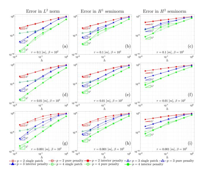
Fig. 3  $L^2$  convergence **a**, **d** and **g**,  $H^1$  convergence **b**, **e**, and **h**, and  $H^2$  convergence **c**, **f** and **i**, associated with the Kirchhoff plate shown in Sect. 5.1, for  $\beta = 10^2$  and for different values of the thickness  $\tau$
