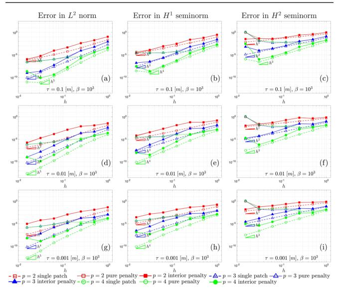
Fig. 9  $L^2$  convergence **a**, **d** and **g**,  $H^1$  convergence **b**, **e**, and **h**, and  $H^2$  convergence **c**, **f** and **i**, associated with the shell shown in Fig. 7a, for different values of the thickness  $\tau$  and arbitrary parameter  $\beta = 10^3$
