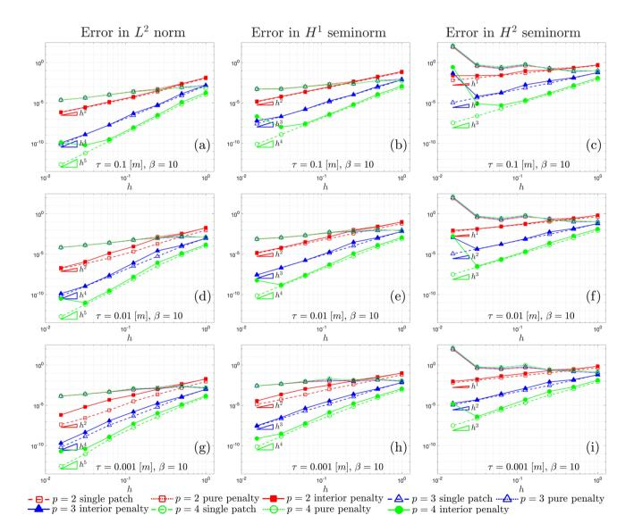
Fig. 8  $L^2$  convergence **a**, **d** and **g**,  $H^1$  convergence **b**, **e**, and **h**, and  $H^2$  convergence **c**, **f** and **i**, associated with the shell shown in Fig. 7a, for different values of the thickness  $\tau$  and arbitrary parameter  $\beta = 10$
