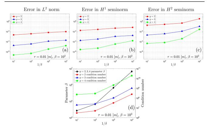
**Fig. 11** Error on  $L^2$  norm (**a**),  $H^1$  seminorm (**b**), and  $H^2$  seminorm (**c**), value of the parameter  $\beta$  (left ordinate in **d**), and condition number (right ordinate in **d**), as functions of decreasing value of the parameter  $\delta$  for the discretization shown in Fig. 10
