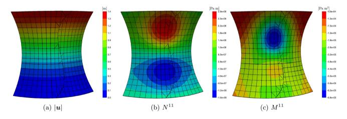
Fig. 12 Undeformed configuration for the shell in Fig. 7a with superimposed mesh grid and contour of the magnitude of the displacement (a), generalized force  $N^{11}$  (b), and generalized moment  $M^{11}$
