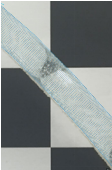
Fig. 6 Manual process in Blender to delineate the contours and extract the 3D mesh of the deformed configuration
