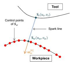
Fig. 7 Definition of the warping vector  $\omega_w^{[k]}$  for a crater to appear on the workpiece
