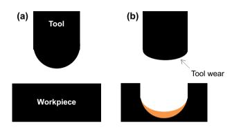
Fig. 2 Tool wear influence in EDM. **a** Tool and workpiece before machining. **b** Tool and workpiece after machining. The *black* workpiece is the desired final profile while the *orange* one is the actual profile that is obtained
