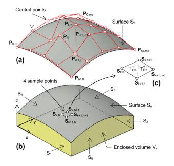
Fig. 6 Enclosed volume computation
