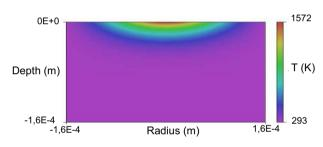
Fig. 4 Temperature distribution from Beck's model
