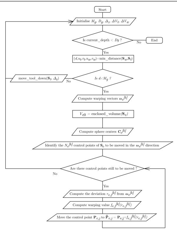
Fig. 5 Flowchart of the simulation's algorithmic process
