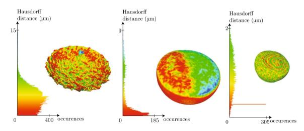
Fig. 16 Hausdorff metric mapped on the meshes of the experimental tool (*left*) and workpiece (*right*). The histogram is displayed on the left of each model
