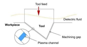
Fig. 1 Principle of EDM
