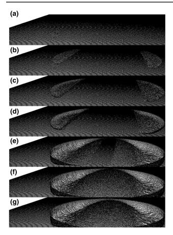
Fig. 11 Evolution of the workpiece's simulated shape: a initial configuration, b 1417 craters, c 24238, d 64543, e 251425, f 285401 and g 374294
