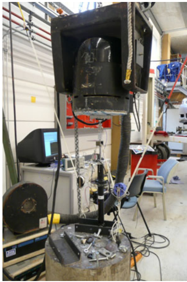
Fig. 15 Damper HIL test setup
